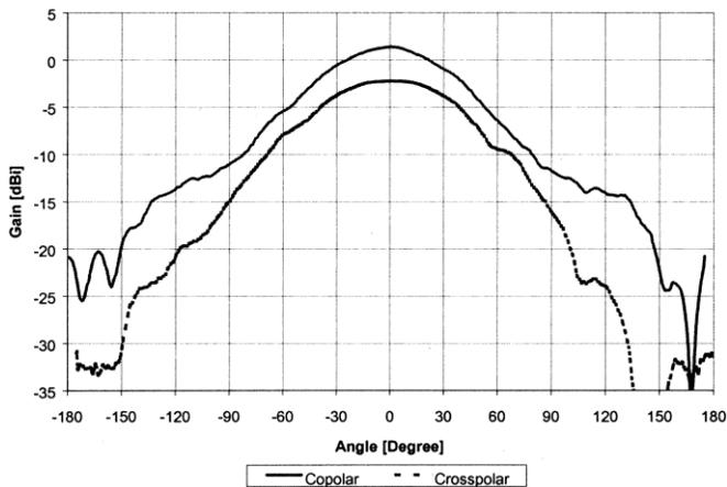
Fig. 4. Experimental E-plane gain.
